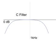
**Filter C** applies C-weighting to your RMS measurements. C-weighted signals are usually indicated by the unit dB(C) or dBC and are based on the 90-phon Fletcher–Munson curve, which means that it refers to the human ear reception on loud sounds. It passes through a broad mid frequency band and attenuates low and high frequencies (see picture).
