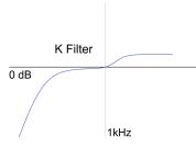
**Filter K** applies K-weighting to your RMS measurements. This filter follows the ITU-R recommendation BS.1770-1 and emphasizes high frequencies above 1 kHz while attenuating low frequencies below 200 Hz (see picture).
