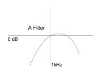
Choose **Filter A** from the dropdown list to apply A-weighting to your RMS measurements. A-weighted signals are usually indicated by the unit dB(A) or dBA. It is based on the 40-phon Fletcher–Munson curve, which means that it refers to the human ear reception on quiet sounds. It emphasizes mid frequencies between 1 and 6 kHz and attenuates low and high frequencies (see picture).
