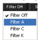
Weighting filters are used for level measurement that is adapted to the frequency weighting the human ear applies at different volumes (according to the so-called Fletcher-Munson curves). Weighted measurement is usually used to judge noise in environments where human beings live or work, but can also be a reference for musical signals. Read more about weighting filters and their meaning in corresponding literature.
