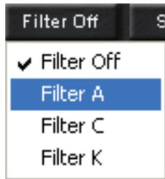
Weighting filters are used for level measurement that is adapted to the frequency weighting the human ear applies at different volumes (according to the so-called Fletcher-Munson curves). Weighted measurement is usually used to judge noise in environments where human beings live or work, but can also be a reference for musical signals. Read more about weighting filters and their meaning in corresponding literature.
