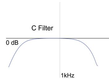
**Filter C** applies C-weighting to your RMS measurements. C-weighted signals are usually indicated by the unit dB(C) or dBC and are based on the 90-phon Fletcher-Munson curve, which means that it refers to the human ear reception on loud sounds. It passes through a broad mid frequency band and attenuates low and high frequencies (see picture).
