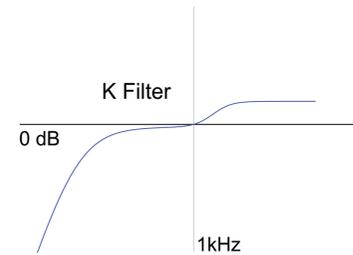
**Filter K** applies K-weighting to your RMS measurements. This filter follows the ITU-R recommendation BS.1770-1 and emphasizes high frequencies above 1 kHz while attenuating low frequencies below 200 Hz (see picture).
