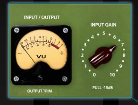
the fixed limiter threshold of the XLA-3. Higher settings of this control will allow the input signal to drive the limiter harder, yielding a stronger compression effect (indicated by the Gain Reduction meter).
