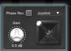
Phase Rev. Matrix Gain Gain -3.2 dB Using the Joystick or Matrix on the interface is a great way to zero-in on a desired character frequency range, without the need to jump back and forth between the LPF and HPF. Once you have found the character you are looking for, adjust the Makeup Gain to compensate for any loss in volume due to filtering. Then, the deeper controls for each filter allow the setting to be tweaked to a point of perfection.
