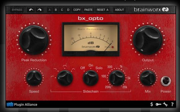
The bx\_opto has a 'Peak Reduction' parameter that increases sidechain gain, while providing a makeup gain parameter to compensate. It also has a 'Speed' knob that affects mostly the release behavior of the compression; clockwise motion speeds up transient response. The bx\_opto also includes a fully sweepable sidechain filter with four different settings and the option to solo. The meter shows accurate gain reduction performed by the compressor.
