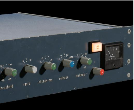
Built in 1978 by the Townhouse maintenance staff from components supplied by Solid State Logic, this is the first outboard SSL bus compressor ever built. The Townhouse Compressor was designed and built to replicate the master buss compressor in an SSL 4000 B console.
