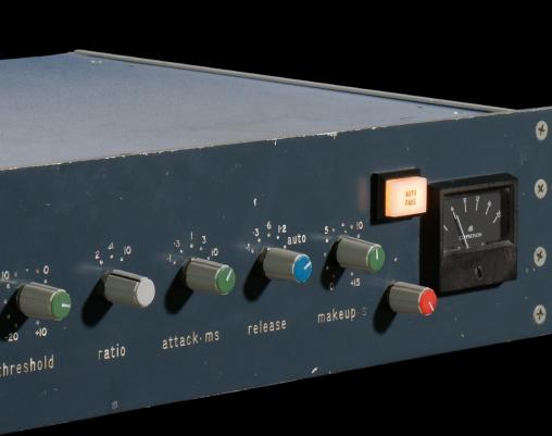
Built in 1978 by the Townhouse maintenance staff from components supplied by Solid State Logic, this is the first outboard SSL bus compressor ever built. The Townhouse Compressor was designed and built to replicate the master buss compressor in an SSL 4000 B console.
