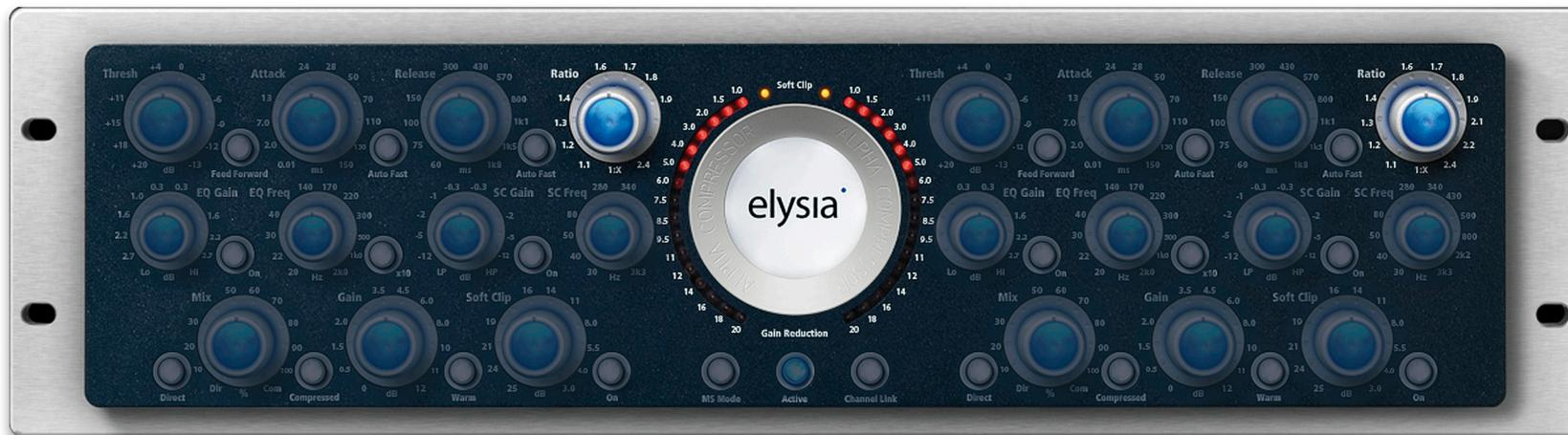
The alpha compressor works with a soft knee characteristic with rising gain reduction values at increasing ratios. The scale on the front panel is based on a measured gain reduction of 6 dB.
