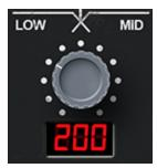
Controls the crossover frequency between the low band and the mid band.
