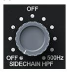
Controls the frequency of the compressor side chain high pass filters.
