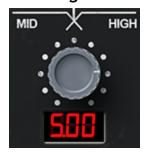
Controls the crossover frequency between the mid band and the high band. When the frequency is displayed in decimal notation, it is in kHz, else it is in Hz.
