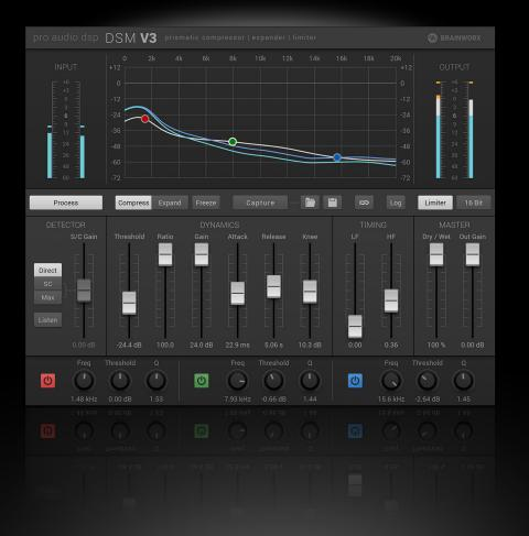
Faster **Attack** and **Release** times can often be used effectively because the action is restricted only to high frequency events.
