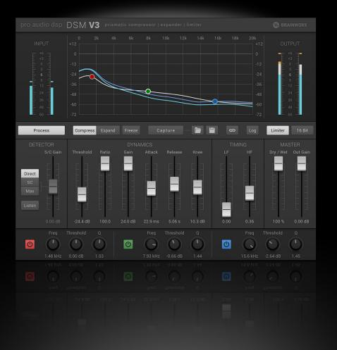
By applying a suitable Threshold spectrum that preferentially compresses the HF content, a useful softening of the high frequency content can be achieved which is reminiscent of tape saturation effects. Some included set-ups illustrate this effect.
