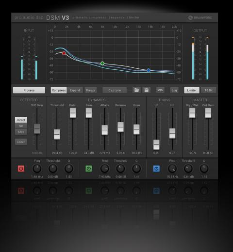
To achieve this, higher overall threshold settings can be used to apply a modified (artificial) threshold spectrum only to the top few dB of the dynamic range.
