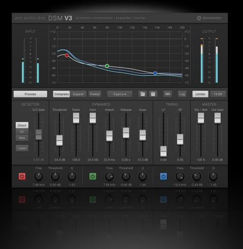
At this point the programme will be effectively gain limited to the response of the captured spectrum. This can be confirmed by toggling the **Process** button to turn the processing on and off, where the processed sound should closely resemble the original programme over the passage where the capture was taken.
