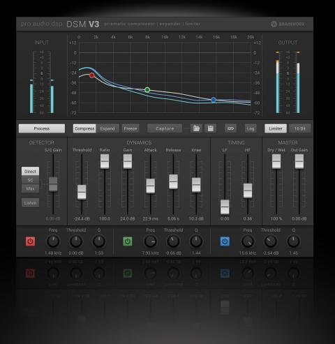
The **Max** setting on the sidechain input section allows the DSM to respond to whichever is the higher signal in any frequency range, which means you can blend the sidechain effect with the direct compression.
