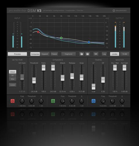
By manipulating the **Attack** and **Release** controls it is possible to cause the voice to blend towards the **Threshold Spectrum** over a period of time without crushing the sibilance. This can be useful for preferentially moderating sustained vocal phrases, particularly when they can often have a tendency to become harsh in many vocal styles.
