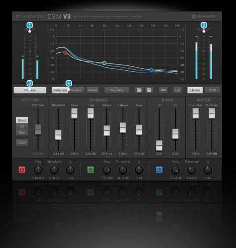
In Compression mode, dynamic gain change can occur anywhere on the graph where the blue curves (stereo) or yellow curve (link Mode on) is higher than the white threshold curve. Where the blue or yellow curve remains beneath the white curve the signal at those frequencies will remain unchanged.
