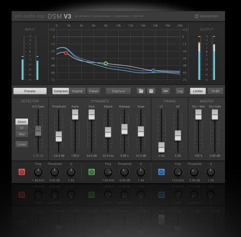
For convenience, the **Ratio** control settings for compress and expand are treated and saved separately, so you can switch between them without loss of settings.
