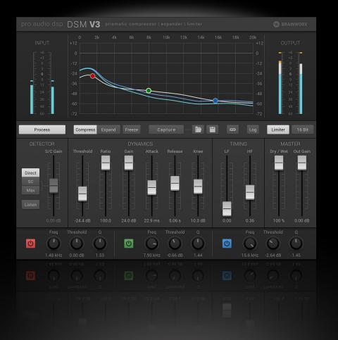
The timing controls act in the same way as a conventional compressor. Increasing the **Attack time** will slow response to peak events, reducing the **Decay time** will speed up gain recovery after compression events.
