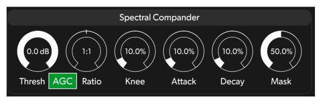
After all of the Effects are applied, the signal runs through the Spectral Compander. Unlike a typical compander (compressor + expander), *every single frequency bin* has its own compander. This means that if you have an FFT size of 1024, there are 1,024 separate companders running inside of SpecOps simultaneously!
